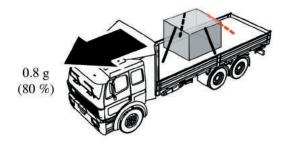
To counteract forward movement, attach the tiedown so it pulls the cargo toward the rear of the vehicle.
