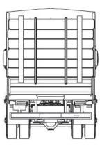
Acceptable securement of one stack loaded crosswise
