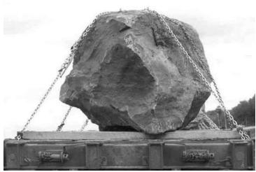
Chain is used to secure large boulders
