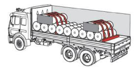
No paper rolls in second layer unless bottom layer extends to front of vehicle
