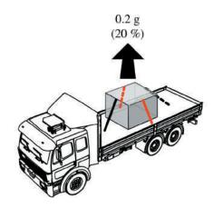
To counteract upward movement, attach tiedowns to opposing sides of the cargo so they pull the cargo down.
