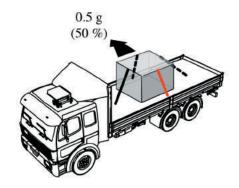
To counteract movement to one side, attach the tiedown so it pulls the cargo toward the opposite side of the vehicle.
