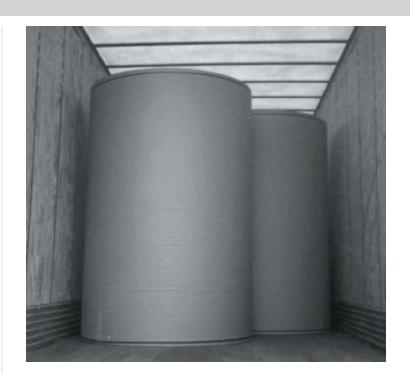
Special Circumstances: Loading and Securing Paper Rolls with Eyes Vertical in a Sided Vehicle (Section 3.4.2) (continued)
